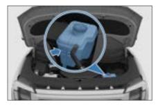
Motor controller coolant expansion tank
