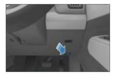
2. Raise the hood to an appropriate height; then it will automatically rise to the open state.
