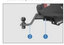
2. Insert the bolt ① into the hole, and then insert the bolt lock ② into the bolt. To assemble the bolt lock as shown in the illustration.
