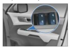
Driver's side power window: Press all the way down and release the switch to open the window. Lift all the way up and release the switch to close the window. Press the switch again to halt the current action.
