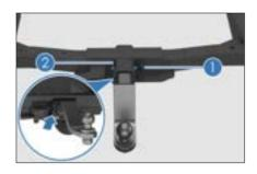
3. Check that the hitch is firmly inserted into the square hole receiver. Try pulling down on the hitch to confirm that the hitch does not drop.
