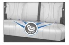
The outboard rear seats are equipped with top tether strap anchorages on the rear bulkhead, behind the rear seat.
