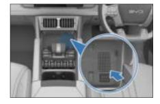
· Wireless phone charging uses a coil to transmit electrical energy to a phone
