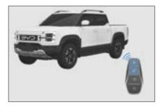
If a door, the hood or the tailgate is not closed, the turn signals do not flash, and the horn sounds once.
