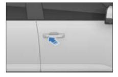
If a door, the hood or the tailgate is not closed, pressing the microswitch will still lock the closed doors, but the horn will only sound once, and the turn signals will not flash.
