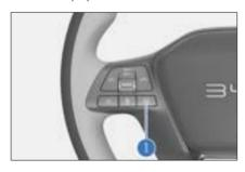
· Enable or disable ICC in the infotainment touchscreen → 🖨 → ADAS → Driving Assist. This function can only be disabled on the infotainment touchscreen when the vehicle is in "P". When the vehicle is started, the system defaults to previous settings.
