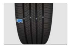
Wear marks are cast inside tire treads. When the tread is worn at this point, a
