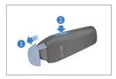
Press the "PUSH" button and insert the mechanical key back into the smart key when it is not in use.
