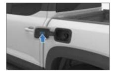
The charging warning label is attached on the upper part of the inner side of the charge port door.
