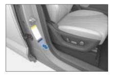
The child protection lock label is engraved on the metal sheet surface on the left/right rear door.
