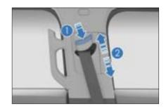
5. Pull the shoulder belt firmly to check that the adjuster is locked.
