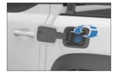
3. After refueling, screw up the fuel tank cap clockwise and then close the fuel door
