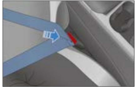
4. The height of the front seat belts can be adjusted for optimum comfort and protection.
