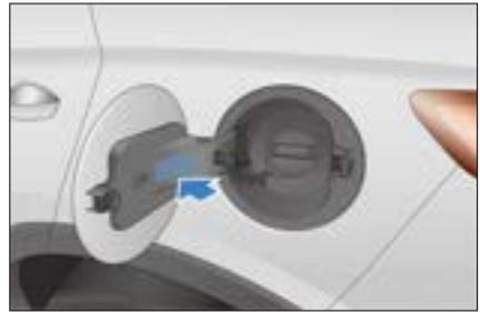
The warning label of the charging port cover is pasted on the inner side of the charging port cover.
