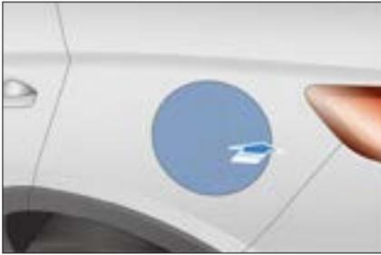
2. Press the refueling button. The instrument shows pressure releasing and reminds that please refuel after 2s. Then press the fuel filler hatch to open it.
