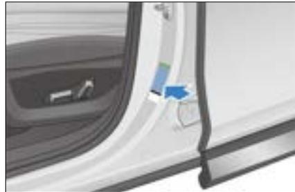
The tire pressure label is attached to the sheet metal surface of the right B-pillar door frame.
