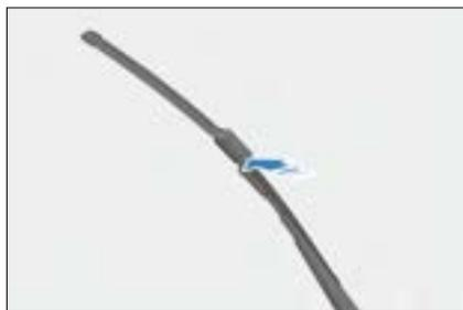
3. Hold the wiper blade clip and take out the wiper blade in the direction shown in the figure.
