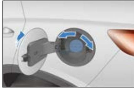
5. If the fuel filler cap has been left open for a long time and you need to refuel, close the fuel filler cap, then press the fuel filler button and follow the step ② to refuel.
