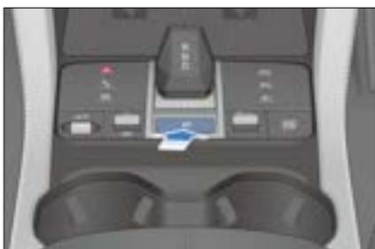
The transmission can be shifted to D/R only when the ignition is on.
