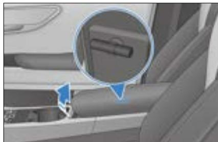
4. Hold the handle firmly, hold the hammer end against the glass, push against the glass to activate the spring release.
