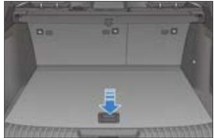
In-Vehicle tools includes: warning triangle, reflective vest, removal clamp for wheel nut cap, jack rocker wrench, towing hook and so on.
