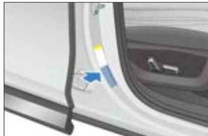
The battery position label is attached below the left B-pillar.
