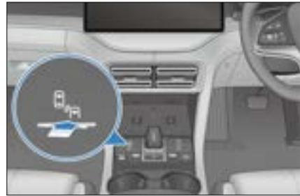
When the blind spot assist system is disabled, no relevant indicators are displayed on the cluster.
