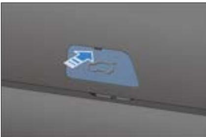
2. Pull the pull lever ①\*/lock ②\* to unlock the boot lid.
