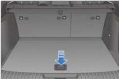
2. When installed at the lower height position, the boot cover board is stuck on the lower step surface of the support plate, and the storage space can be enlarged.
