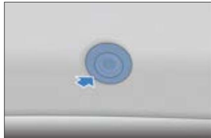
When the vehicle power is not OFF and the "DOOR" switch is turned on, if this switch is pressed with the door open, the interior light switches from high to low light, and does not go out. When the vehicle is powered off and the "DOOR" switch is turned on, the light goes out after a period of time if the door is opened. If there are other operations during the period, it is timed again. (The
