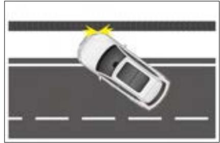
Parts other than the passenger compartment receive side impact.
